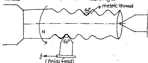
It is a continous form of helical ridges Produced over a Cylinder or Frustum Externally or Internally used for motion transmission and fastening two objects.
